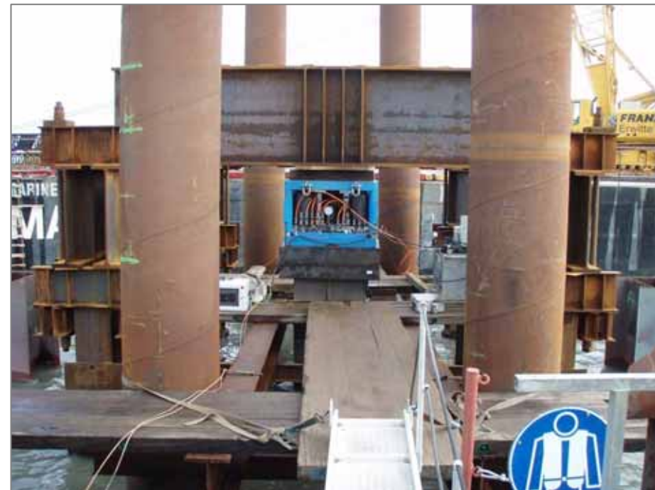
Load bearing test: compression
