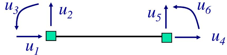
$$\mathbf{K}_{EB-beam} = \begin{bmatrix} \frac{EA}{L} & 0 & 0 & -\frac{EA}{L} & 0 & 0 \\ 0 & \frac{12EI}{L^3} & \frac{6EI}{L^2} & 0 & -\frac{12EI}{L^3} & \frac{6EI}{L^2} \\ 0 & \frac{6EI}{L^2} & \frac{4EI}{L} & 0 & -\frac{6EI}{L^2} & \frac{2EI}{L} \\ -\frac{EA}{L} & 0 & 0 & \frac{EA}{L} & 0 & 0 \\ 0 & -\frac{12EI}{L^3} & -\frac{6EI}{L^2} & 0 & \frac{12EI}{L^3} & -\frac{6EI}{L^2} \\ 0 & \frac{6EI}{L^2} & \frac{2EI}{L} & 0 & -\frac{6EI}{L^2} & \frac{4EI}{L} \end{bmatrix}$$
